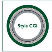
Style CGI, Similar to a CG gasket but fitted with inter ring giving additional compression limitation and providing a heat and corrosion barrier, protecting windings and preventing flange erosion.
