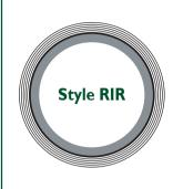
Style RIR fitted with a solid inner metal ring acting as a compression stop, fills the space between flange bore and ID of the gasket. Prevents accumulation of solids, reduces turbulent flow and minimizes erosion at flange faces.
