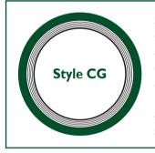
Style CG fitted with an external ring which accurately centers gasket on the flange face, provides additional radial strength preventing gasket blow-out and acts as a compression stop.
